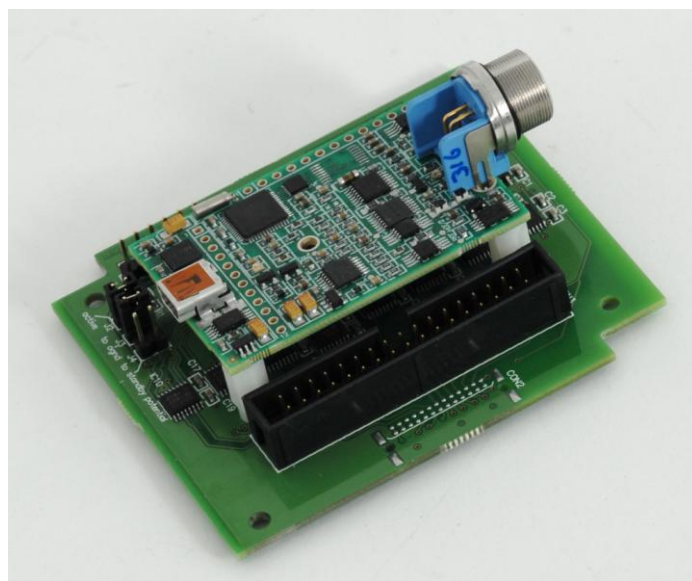
Printed circuit boards of the EmStat/Mux with USB connection.
