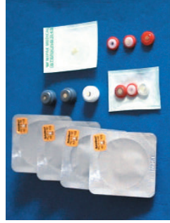
Membrane type biosensors – for application in glucose and lactate analyzer
