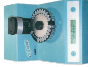
eco twenty / Care diagnostica Glucose analyzer based on thick film technology
