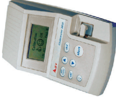
Glukometer 3000 ® BST GmbH Mobile glucose system for POCT application
