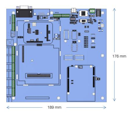
Max. height without shielding can, without standoffs: 25 mm
