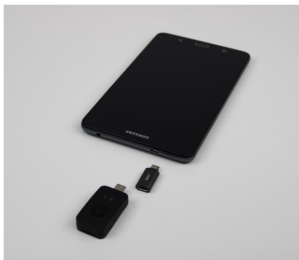
Figure 1.1 The Sensit Smart with a Galaxy Tab A and the USB-C to micro USB converter
