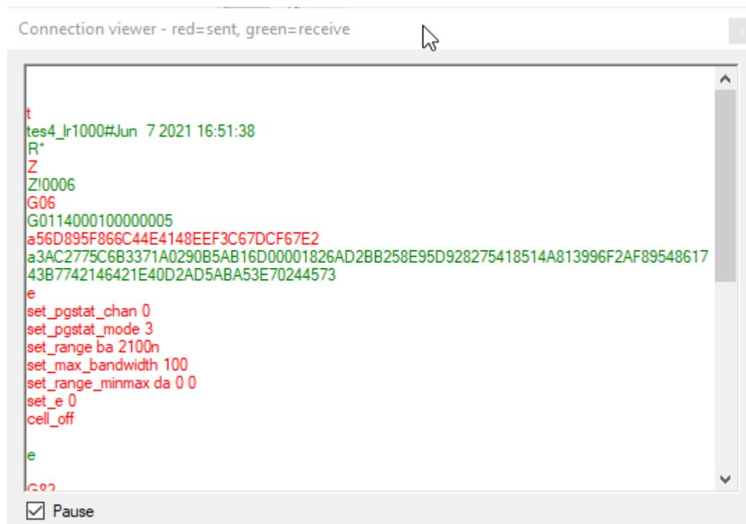
The connection viewer window. All information in red is sent from the PC to the device and the green information is sent by device to the device.
