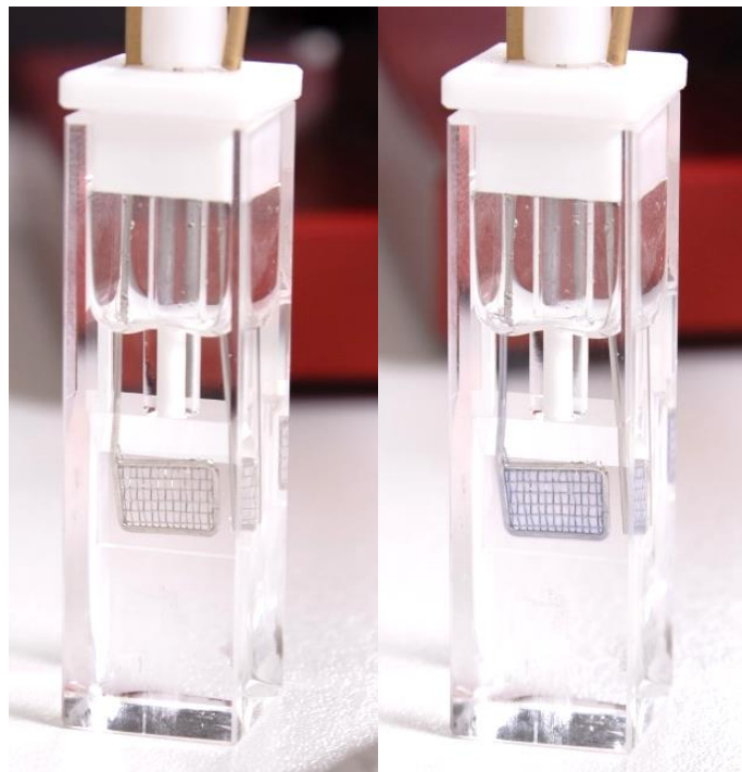
The platinum mesh changes color by applying a voltage. What if you could measure the change with a spectrometer?
