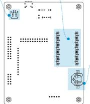
RTC Battery Compartment CR1220 3V Real Time Clock backup source
