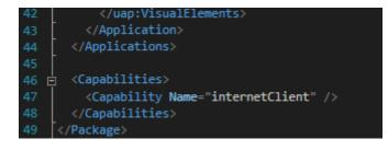
To use an Emstat device in VCP mode add the following code to the capabilities:
