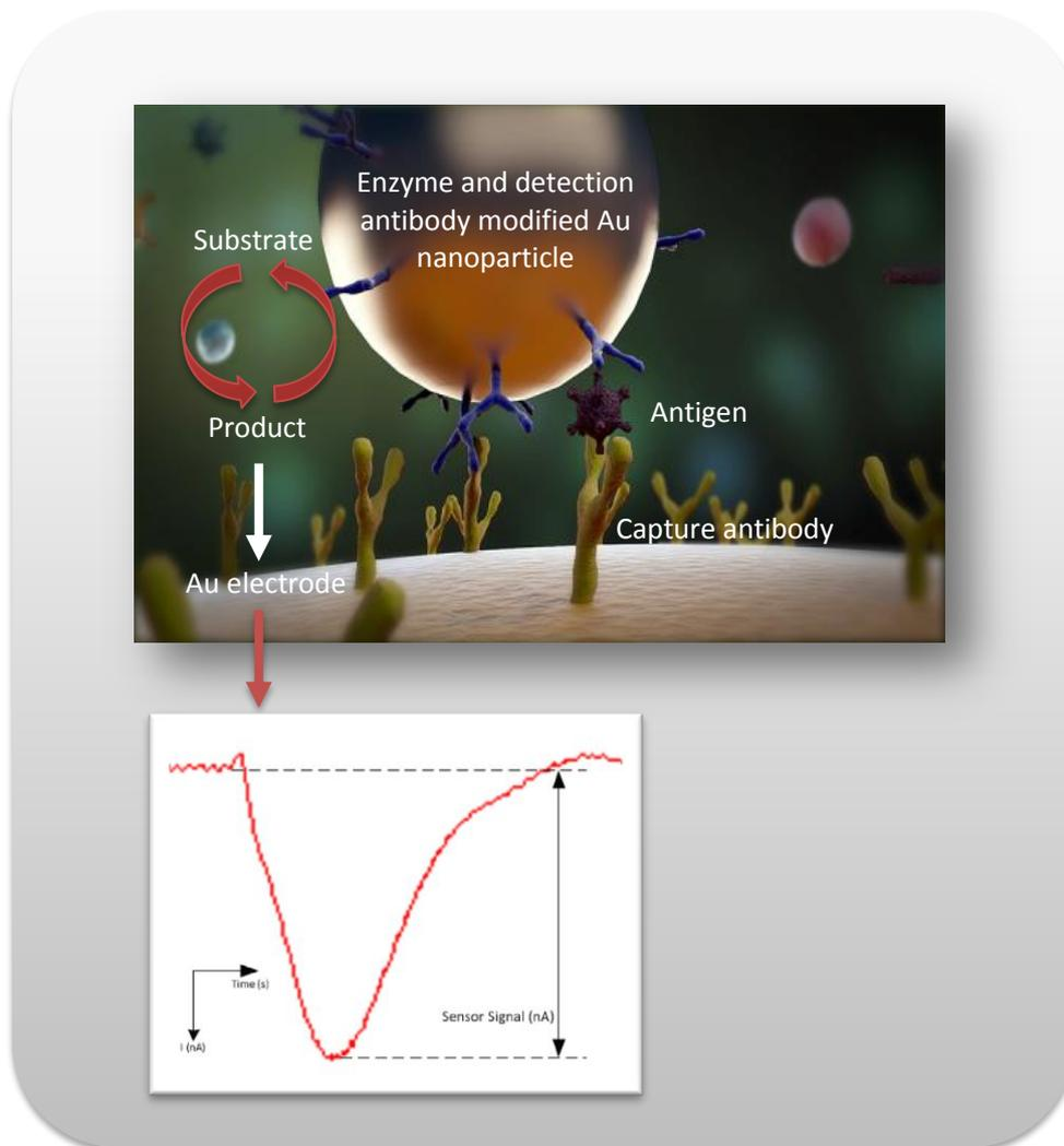
Figure 1. Detection Mechanism and results
